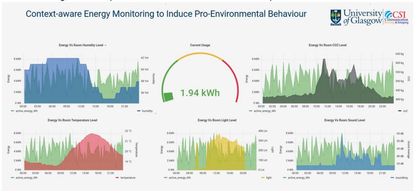
Figure 1: The Energy Dashboard Displaying Consumption vs Environmental Parameters
